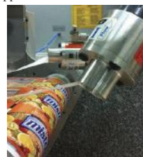
1" (25mm) Line Vac removes and discards a label matrix.
